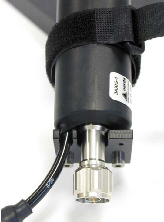
Figure 6: Cable and N connector in guideway
