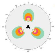
Example: side-view of directional antenna (vertical, or elevation, pattern)
